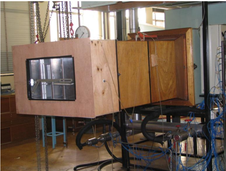
Figure 1.2 Ventilator connected to draft tunnel
