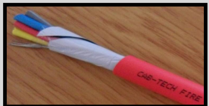
Cable print: CAB-TECH FIRE 1.5 MMSQ 4 CORE FIRE RESISTANT CABLE BS EN 50200 & BS 8434-2 PH120 ENHANCED / SANS 10139(B/NO)
