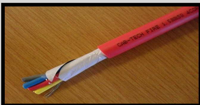
Cable print: CAB-TECH FIRE 1.5 MMSQ 4 CORE FIRE RESISTANT CABLE BS EN 50200 PH30 STANDARD / SANS 10139 (B/NO)
